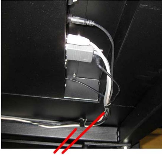
Cable clamps can be installed under platform to enable cables to be neatly secured
